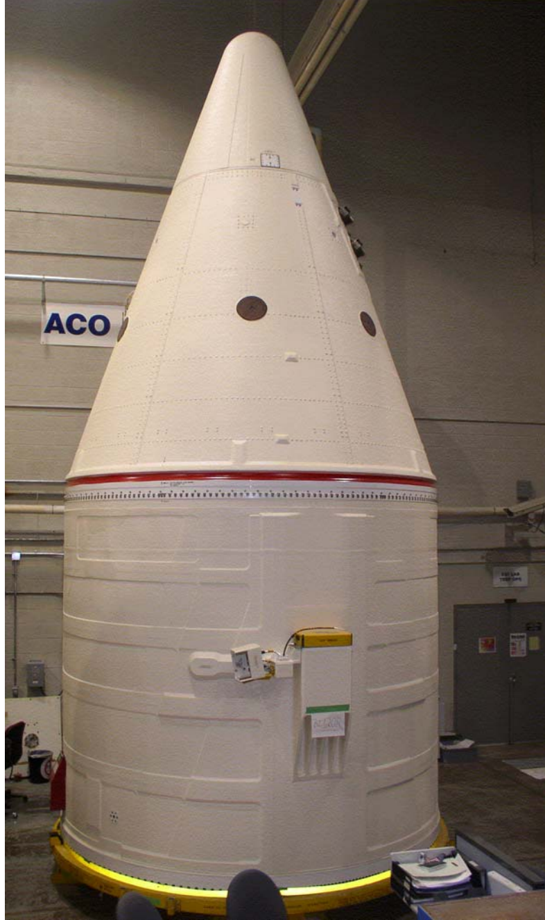
SRB Forward Assembly (Nose Cap, Frustum, Forward Skirt)
